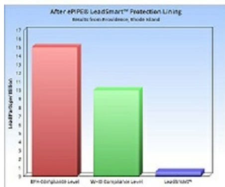
Post ePIPE Lining Results in Providence: Lead leaching less than 1 ppb when tested internally
